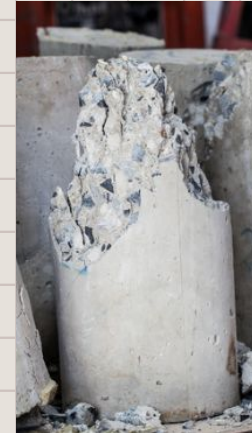
Figure 24: Ideal cylinder break
