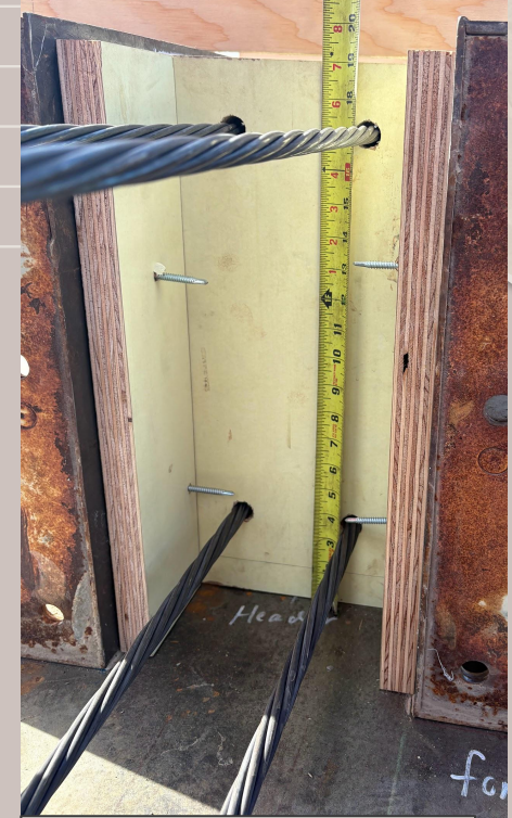
Figure 18: Verification of strand measurements
